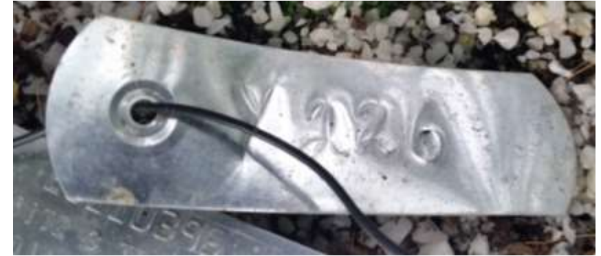
Additional unique label: engraved by hand into soft aluminium
