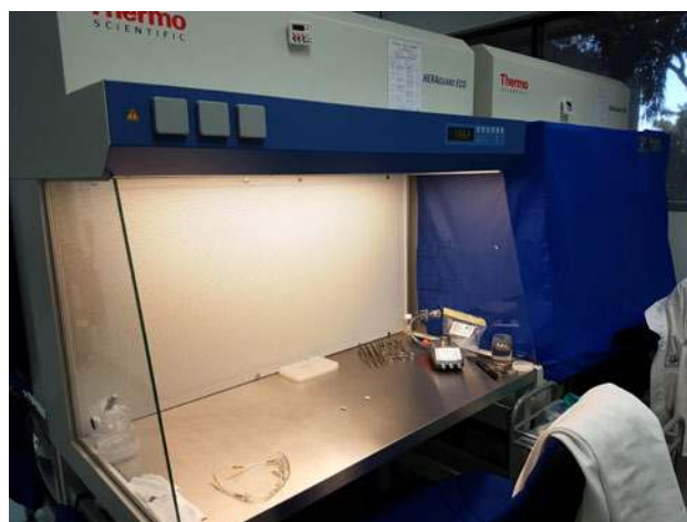
Figure 11. A laminar flow cabinet for sterile work. (Photo: L. Commander)
