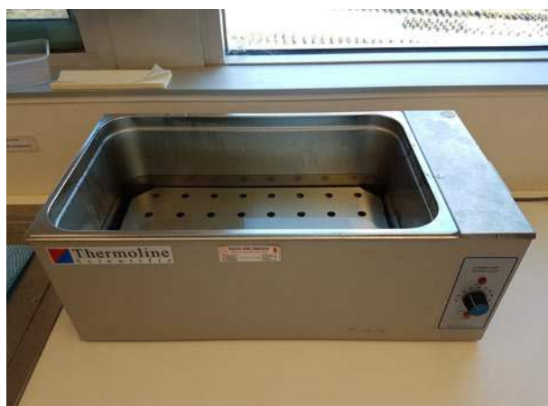
Figure 15. A hot water bath used for treating seeds with physical dormancy. (Photo: L. Commander)
