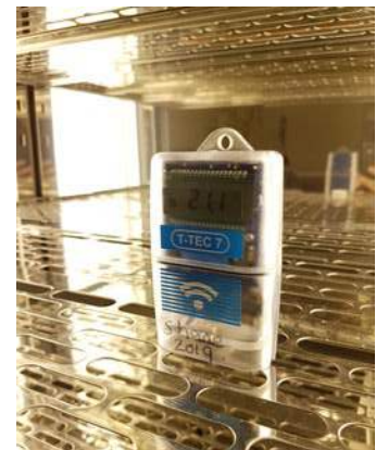
Figure 5. A small datalogger can be used to record temperatures during incubation of germination tests, either within a cabinet or within a room. (Photo: L. Commander)
