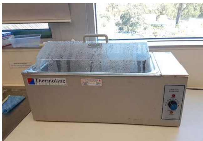
Figure 15. A hot water bath used for treating seeds with physical dormancy. (Photo: L. Commander)
