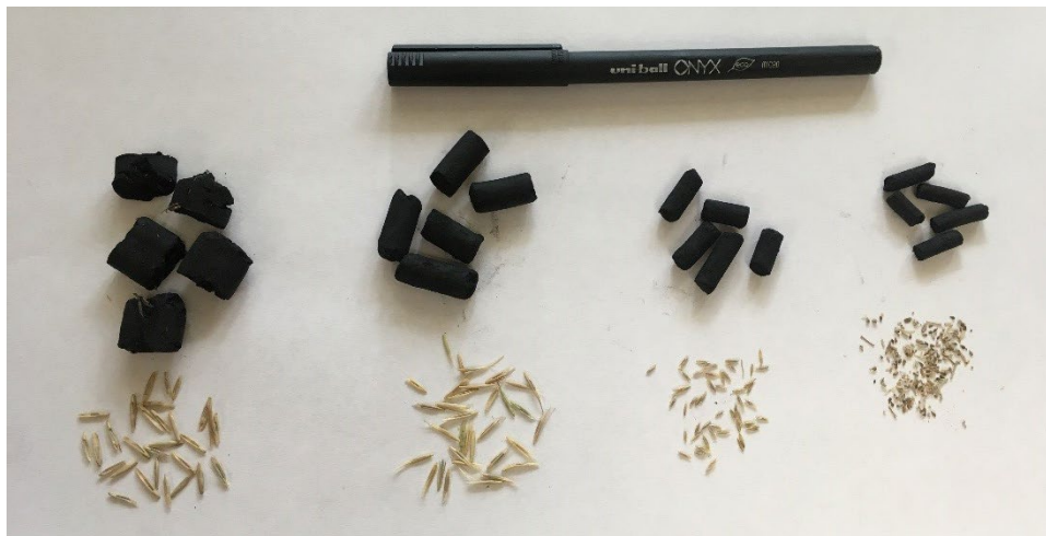
Figure 6. The extruded pelleting process begins with a mixture of organic, inorganic materials, seeds and water that make up the “dough” (top left images) which forms the extruded pellets. The dough is placed into the extruder unit (a wet-extrusion, pasta-style unit shown here; top middle), which produces extruded pellets that can be laid out on a flat drying tray and dried at constant conditions (e.g. ca. 25-40°C with a forced air drier; top right) prior to use or storage. The pellet dimensions and number of seeds per pellet are easily customisable to ensure optimised embedding of seed (see recent examples in Baughman et al. 2021; Ritchie et al. 2020; Stock et al. 2020). (Photos: V. Brown and O. Baughman)
