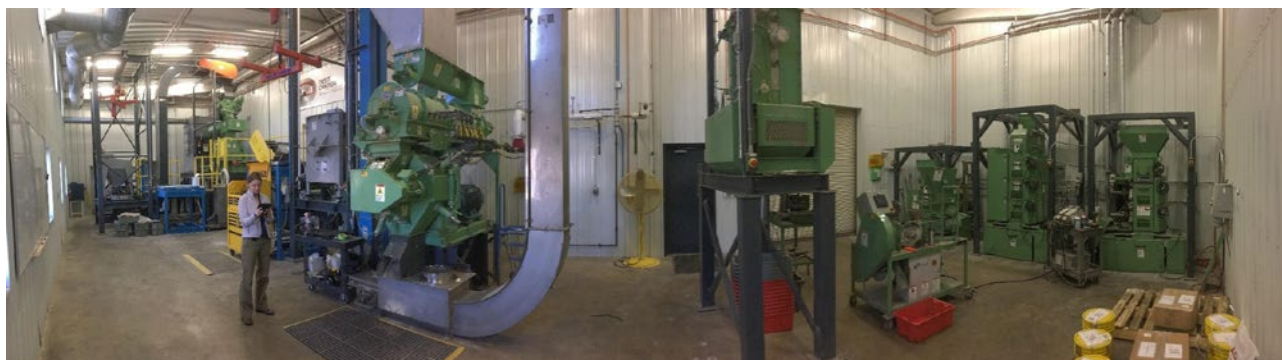
Figure 7. Example of a commonly used industrial pelletizing mill and drying unit used for small-scale industrial applications, capable of producing \geq 2 tonnes per hour. Larger sizes are also common. Use of such mills to produce SETs is in its infancy but the customisability and scalability offered is promising. (Photo: O. Baughman)
