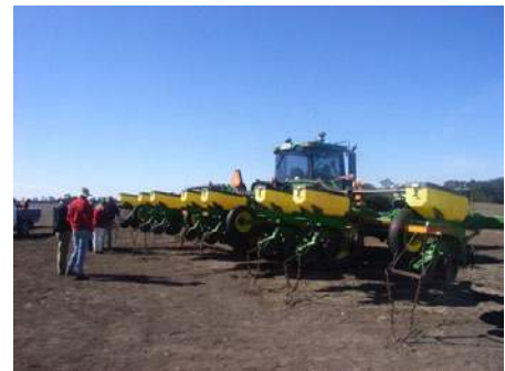
Figure 7. Various types of agronomic air-seeders able to apply cleaned and flowable seed at large scales. (Photos: D. Carr)
