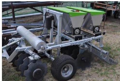
Figure 7. Various types of agronomic air-seeders able to apply cleaned and flowable seed at large scales. (Photos: D. Carr)
