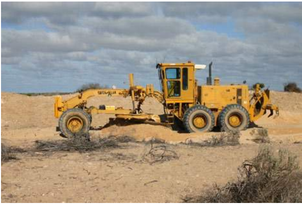
Figure 4. Large machinery such as graders can be used for site preparation including ripping, especially at mine sites and quarries. (Photo: L. Commander)
