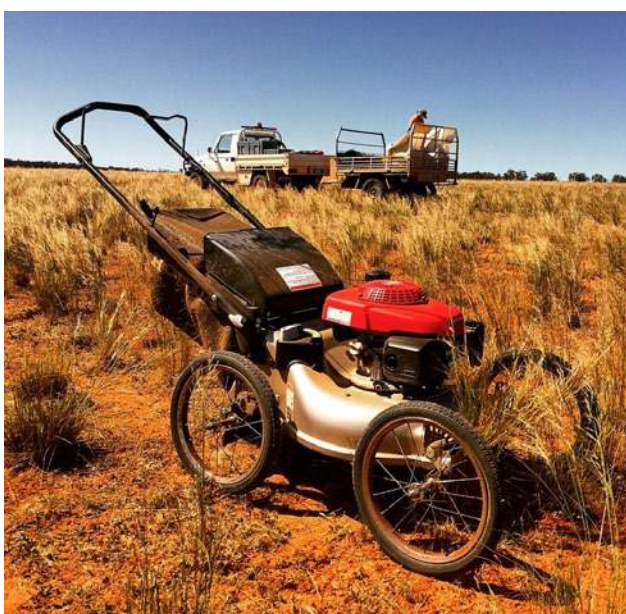
Figure 9. An adapted lawn mower with BMX wheels. (Photo: T. Zwiersen)
