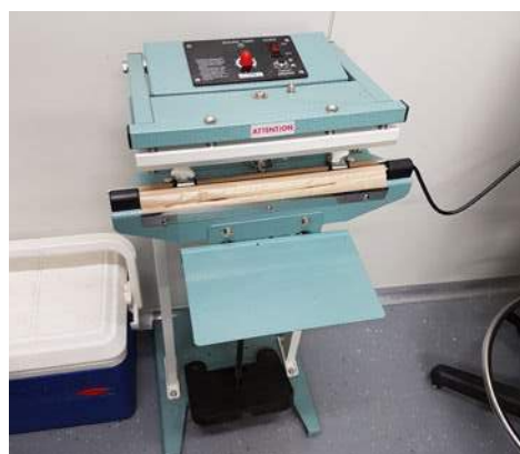
Figure 7. Benchtop (left) and foot operated (right) heat sealer for sealing plastic or foil bags. (Photos: L. Commander)
