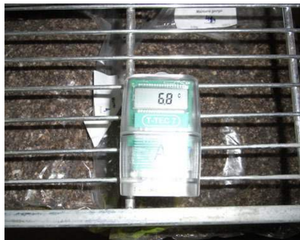
Figure 14. A data logger can be used to display and record temperature and humidity in the seed store as well as during pre-storage drying. (Photo: L. Commander)
