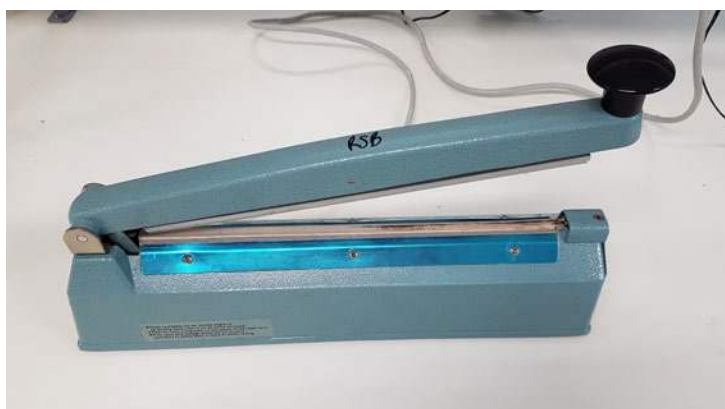
Figure 7. Benchtop (left) and foot operated (right) heat sealer for sealing plastic or foil bags. (Photos: L. Commander)
