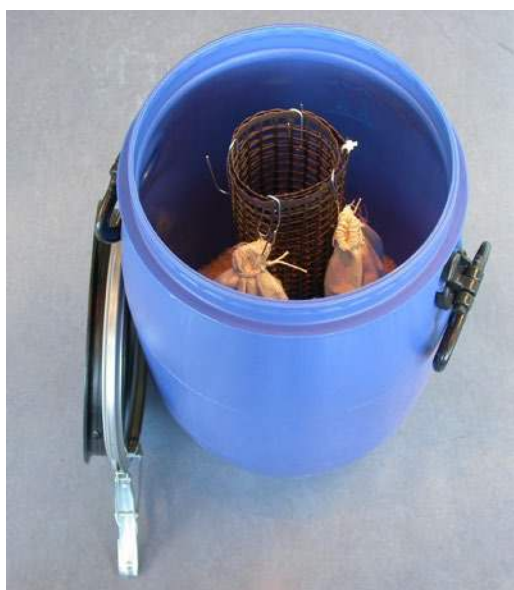
Figure 5. Silica gel drum dryer containing seeds (left) and containing a hygrometer (right). (Photos: RBG Kew)
